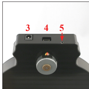
3- Power input; 4- USB socket; 5- Motor tension adjustment
